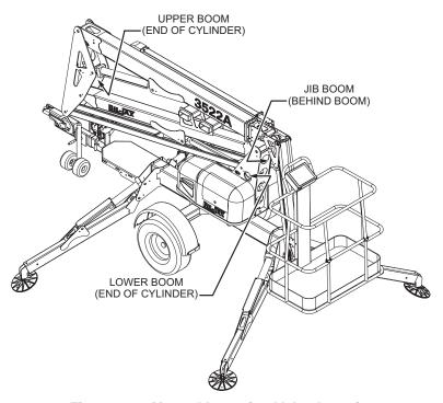
Figure 3-7. Manual Lowering Valve Locations
